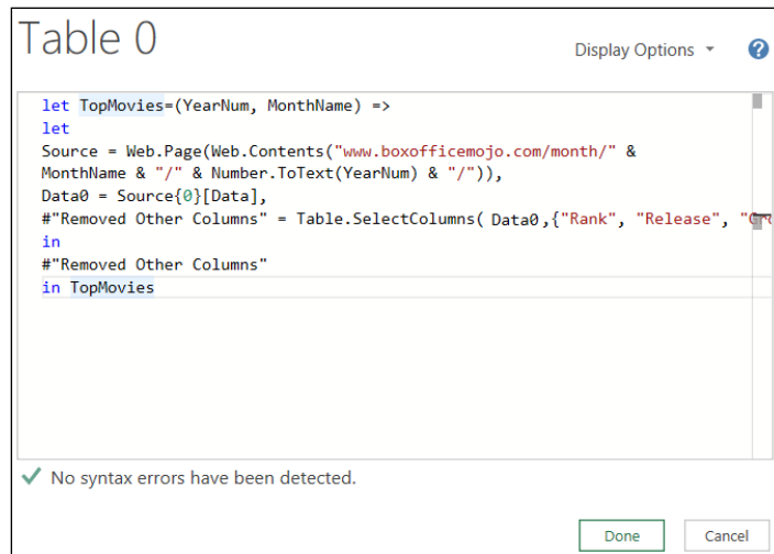
FIGURE 12-19: Wrapping the starter code with function tags and specifying a YearNum parameter and a MonthName parameter.
